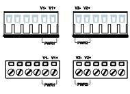
STEP 1: Insert the negative/positive DC wires into the V-/V+ terminals, respectively. STEP 2: To keep the DC wires from pulling loose, use a small flat-blade screwdriver to tighten the wire-clamp screws on the front of the terminal block connector. STEP 3: Insert the plastic terminal block connector prongs into the terminal block receptor, which is located on the IE-SW-PL16M top
