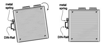
To remove the IE-SW-PL16M switch from the DIN-Rail, simply reverse Steps 1 and 2 above.
