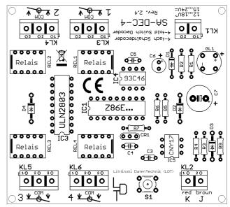
**Remarks:** The decoder addresses for magnet accessories are combined in groups of four. The address 1 to 4 build the first group. The address 5 to 8 build the second group etc. Each **SA-DEC-4** decoder can be assigned to any of these groups. Which of the 4 turnouts of a group will be activated for the addressing does not matter.
