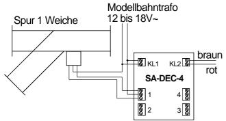
Feed the SA-DEC-4 via clamp KL1 witch AC from the model railway transformer. Further connect one ac-cable of the transformer with clamp 'L' on the turnout drive. Connect the second cable of the transformer with the clamp marked 'COM'
