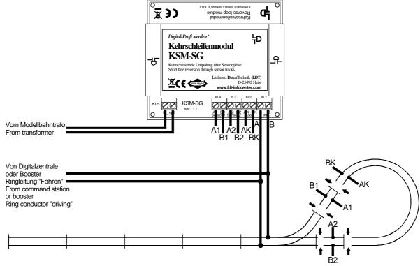
Sample Connection 2: Reverse-loop polarity via the reverse-loop module KSM-SG plus track occupancy report at the reverse-loop with the RM-GB-8-N. Sensor tracks will be monitored as well.
