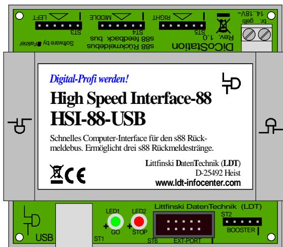
Transmits the feedback information directly to the PC without any detour from the s88 bus via the digital central unit.
