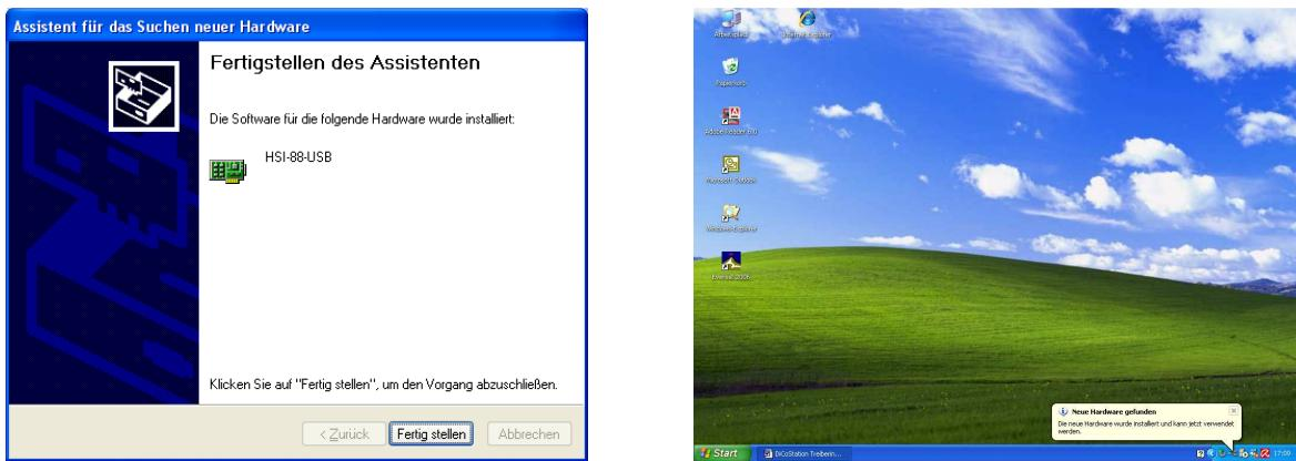
**10.** The installation of the **USB-Drivers** has now been completed. Now you can remove the **CD “USB-Drivers for DiCoStation and HSI-88-USB”** from the **disk drive**.
