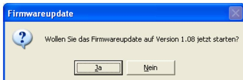
7. During the updates should be the **USB-connection** to the **HSI-88-USB** **not interrupted**. After a short **transmittance time** which will be indicated at two additional windows please **click** under the report **“Firmwareupdate erfolgreich abgeschlossen”** (“Firmware update successful completed”) on **“OK”**.
