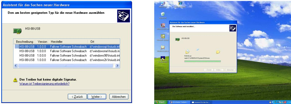
**9.** Click now again on “**Fertig stellen**” (“Complete”) (**image left**). The **PC reports** now that the **new hardware has been installed and can be used** (**image right**).
