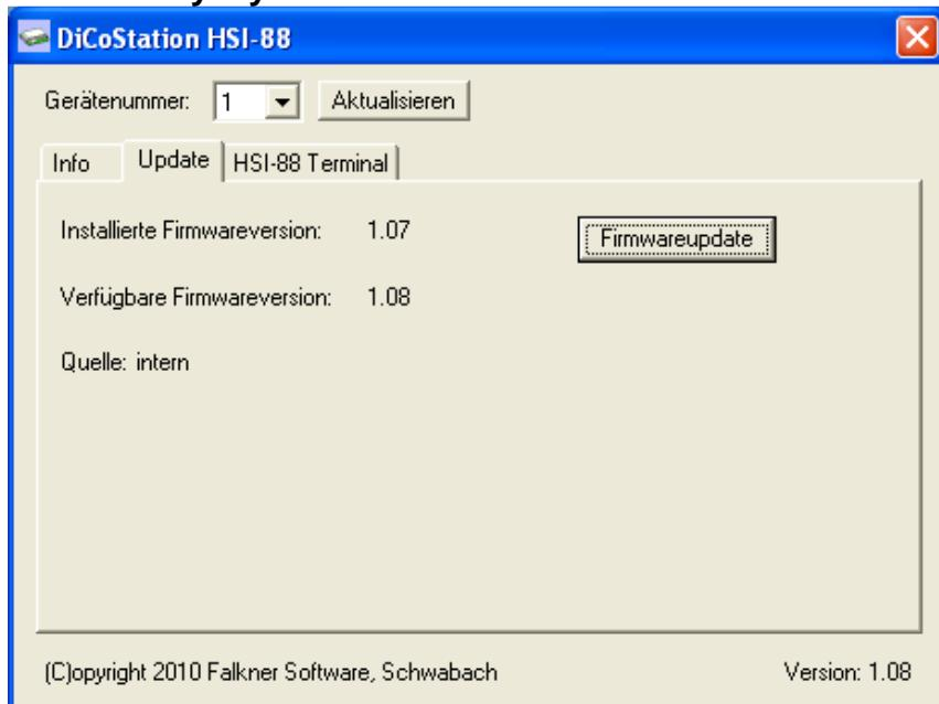
**Important Information:** The **device number** should **never be changed**. Otherwise the model railway software will not **recognize** the **HSI-88-USB** any more. The device number will be important as soon as you use more than one **HSI-88-USB** or **additionally a DiCoStation for driving and switching**. The first **HSI-88-USB** will get automatically always the **device number 1**.
