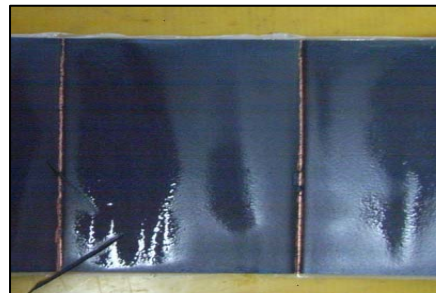
Normal Negative Electrode: Active Material Exfoliation
