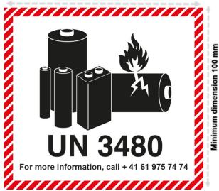
The Lithium Battery Mark (see above) may continue to be used until 31 December 2026 to provide a telephone number for additional information (no need to be 24h reachable). Beginning 1 January 2027 the telephone number has to be removed from the label.
