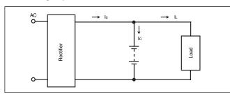
In the above-illustrated model, output current of the rectifier is expressed as:  $I_o = I_c + I_L$  where  $I_c$  is charge current and  $I_L$  is load current. Consideration should be given to secure adequate charging because, in fact, load current is not constant but irregular in most cases.
