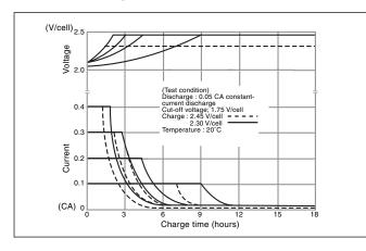
In order to fully utilize the characteristics of VRLA batteries, constant-voltage charging is recommended. For details of charging see pages 19 – 23.
