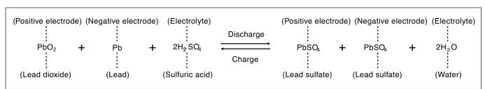
In the final stage of charging, an oxygen-generating reaction occurs at the positive plates. This oxygen transfers inside the battery, then is absorbed into the surface of the negative plates and consumed. These electrochemical reaction processes are expressed as follows.
