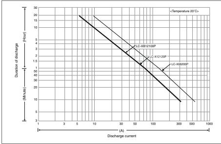
VRLA battery for standby power applications (100Ah)
