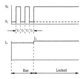
3rd wire signal Run : Square Wave Locked : Vu or Vu
