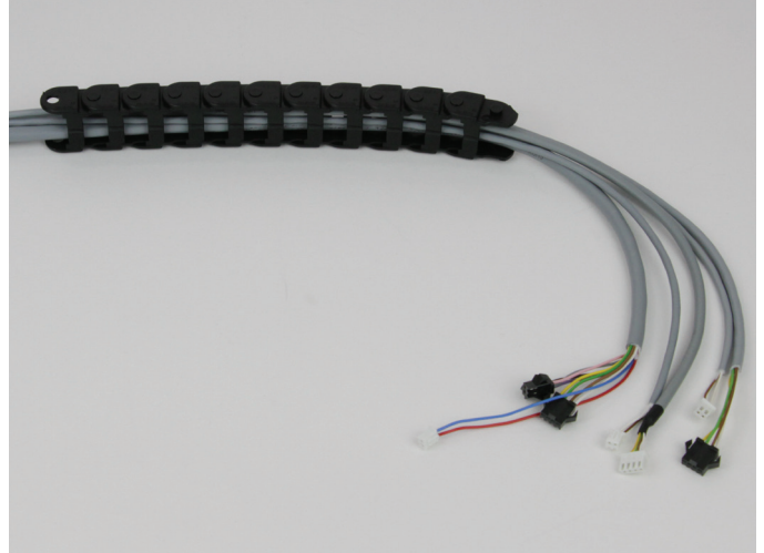
Push the lines into the energy drag chain so that the end link points to the line ends without label (with the number of the line) with the nipples.
