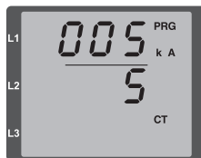
Fig. Current transformer programming mode Use button 1 and 2 to change primary and secondary current (see page 50).
