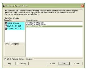
The Utility checks to make sure the KH1508A / KH1516A is in the Firmware Upgrade Mode and then lists all firmware needed preselected in the *Device List* panel.
