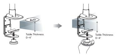
Install Mount with Swivel Arm, Spring Arm, and Monitor Bracket.
