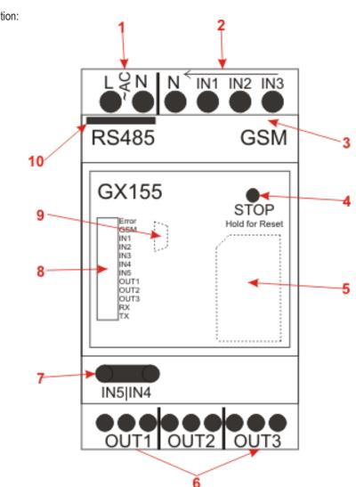
IN1 to IN5 are lit automatically when the input voltage at the input has exceeded the threshold value.
