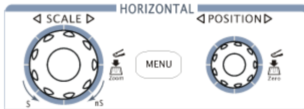
Figure 1-10 The horizontal system
