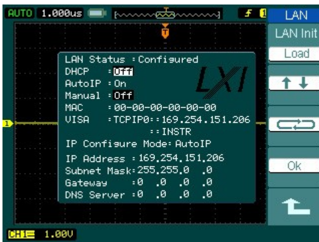
Figure 2-88 LAN Setting interface
