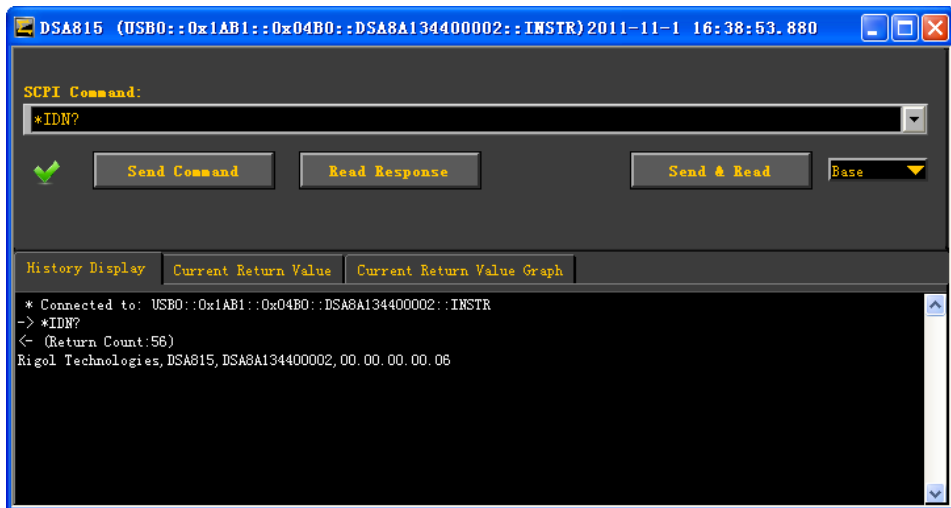
Figure 3-3 Write and Read Commands via USB
