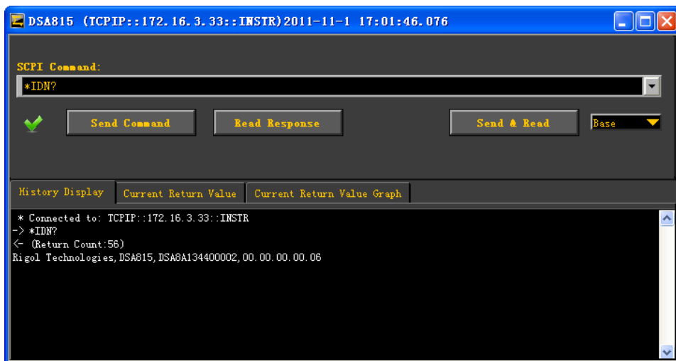
Figure 3-6 Write and Read Commands via LAN
