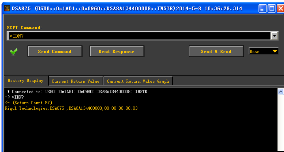
Figure 3-2 Write and Read Commands via USB
