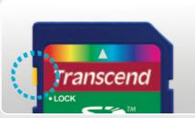
Mechanical write-protection switch
