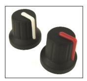
2 colour moulded. 6 standard colours. Soft touch finish. Base Diameter: 16.0 Overall height: 15.0 Shaft depth: 12
