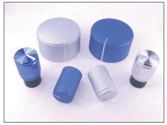
Knobs for professional equipment - comprising machined aluminium shell on moulded plastic inner. Push on fixing. Max shaft depth 11mm.
