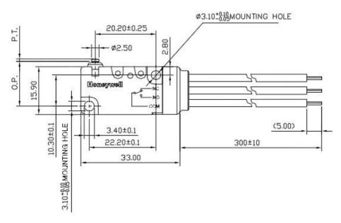
Figure 3. Other MICRO SWITCH™ V15W Series Watertight Miniature Basic Switch Terminal Options
