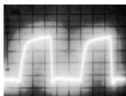
Signal Waveform \left(\frac{20\text{ns/div}}{1\text{V/div}}\right)
