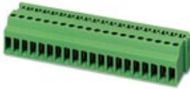
Plug-in card block, Nominal current: 5 A, Number of positions: 20, Pitch: 5 mm, Connection method: Screw connection, Contact surface: Tin
