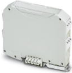
Component housing, Complete housing, Cross connection: DIN rail bus connector, Color: light gray, Width: 17.5 mm, Constructional height: 70.4 mm, Number of positions cross connector: 5
