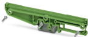
Side element, right, with foot, width: 5 mm wide, length: 122 mm, for mounting on DIN rail NS 32 or NS 35/7.5
