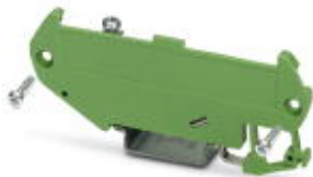
Side element, left, with foot, width: 5 mm, length: 72 mm, for mounting on NS 32 or NS 35/7.5, with PE contact to the DIN rail
