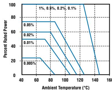
UPW Series resistors must be derated for tolerances below 0.1%. Use the graph to select tolerance versus operating temperature to determine the percentage rated power for operation. No derating is required for operation below 20 °C.
