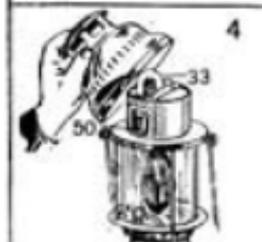
4. Replace the inner Casing and the Hood in good order. The Mixing Tube (33) must aim at the Nipple (50) fitted on the Vaporizer Upper Part (152A) otherwise there will be no emission of light.
