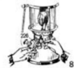
8. Lighting of No. 909 and No. 950 may be effected by Rapid Preheating by lighting Ignition Device (226) and keeping jetting for about 50 seconds.
