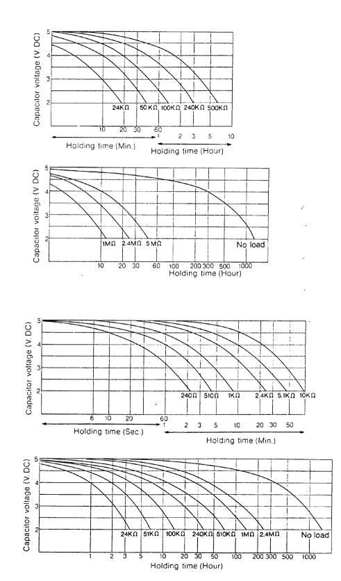
Resistance values vs. charge characteristics (at +25°C)
