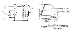
The discharge current shall be caluculated by the capacitance value in a ratio of 1mA/fand.
