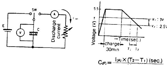
The discharge current shall be calculated by the capacitance value in a ratio of 1mA/fand.
