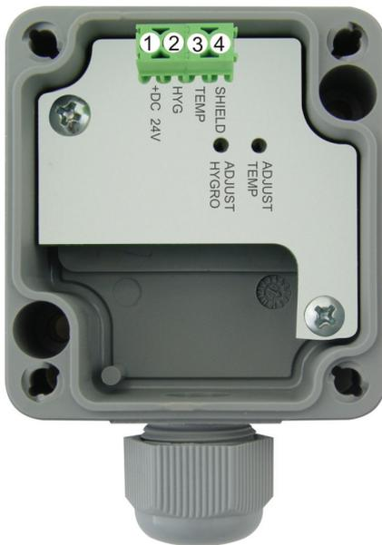
The shielding (SHIELD) is to be optionally covered. Connection through shielded lines is recommended. Operating voltage +DC 24 V is common for both the instrument transformers.
