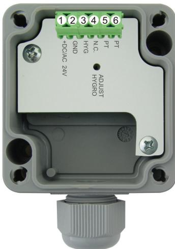
The Pt1000 is with brought out potential free with 3 wire connection. The line resistance is to be compensated. Other types of measuring resistances, for example, NTC resistance, are also possible, if required!
