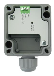
The measurement of the output signal should be done with separate signal ground, in order to avoid measuring error due to voltage drop at the supply ground.
