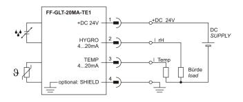
Humidity measurement 4 ... 20 mA and passive Pt1000 for Temperature measurement, Type –TEPT
