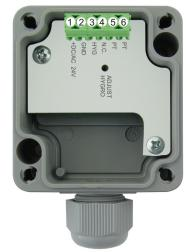
The Pt1000 is with brought out potential free with 3 wire connection. The line resistance is to be compensated. Other types of measuring resistances, for example, NTC resistance, are also possible, if required!
