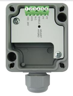
The shielding (SHIELD) is to be optionally covered. Connection through shielded lines is recommended.
