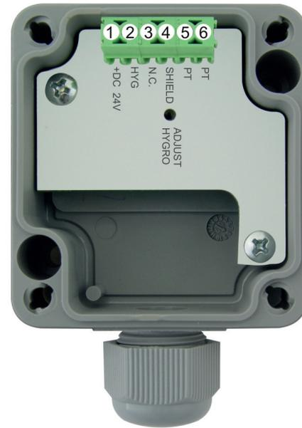
The shielding (SHIELD) is to be optionally covered. Connection through shielded lines is recommended. The Pt1000 is with brought out potential free with 2 wire connection. The line resistance is to be compensated. Other type of measuring resistances, for example, NTC resistance are also possible, if required!
