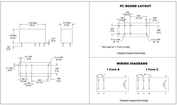
Dimensions in inches with metric equivalents in parentheses. Tolerance: ± .010"
