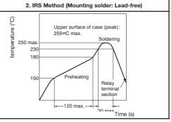
Note: The temperature profile indicates the temperature of the relay terminal section.
