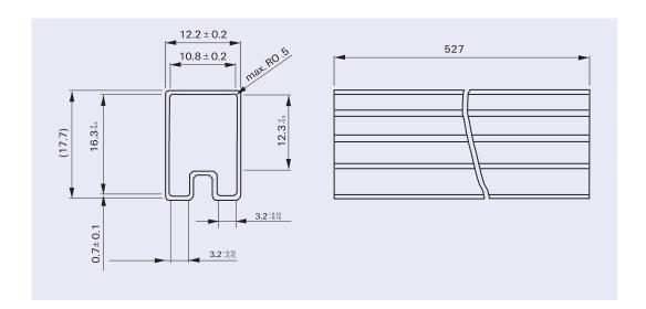
Tube for THT version 25 relays per tube 1'000 relays per box
