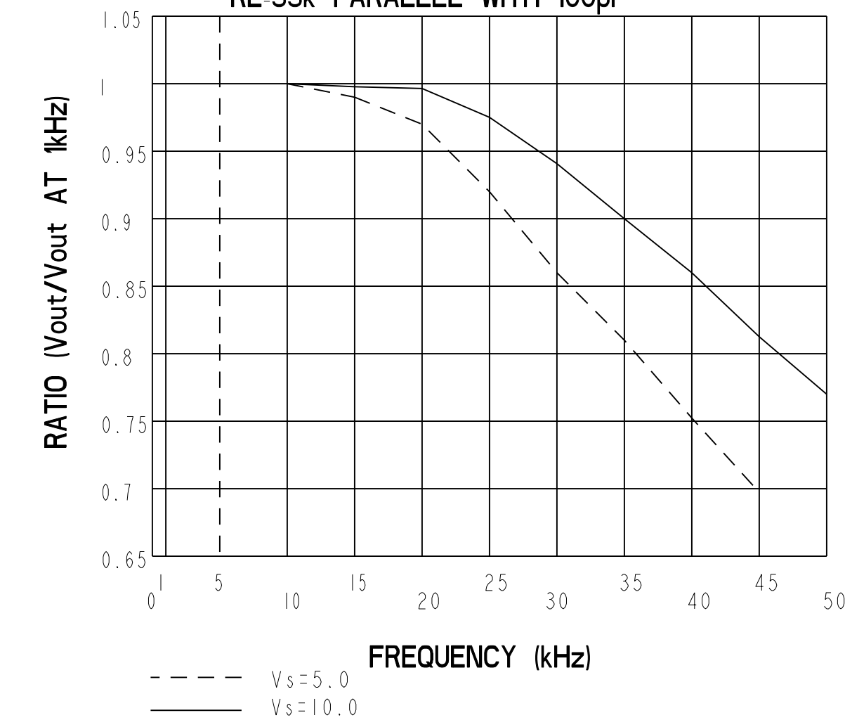
TYPICAL FREQUENCY RESPONSE RL-33k PARALLEL WITH 100pF
