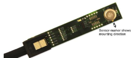
Place the sensor as described above into the adapter board and then connect it with the help of connection leads provided with the PC-adapter.
