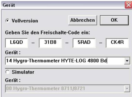
Now for the "Device", select the device driver "14 Hygro-Thermometer HYTE-LOG 4800 BD". The activation code will be registered automatically. Confirm the dialogue with 'OK'.
