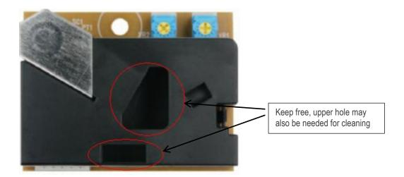
In addition, please pay attention to structure and placing location of the application to avoid any adhesive particles (such as oil, etc) getting into the module, which may cause malfunction by sticking to the optical part.
