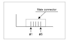
Control (Pin #1) This pin is used for tuning the sensitivity when Vout1 is used.
