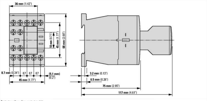
Contactor with auxiliary contact module
