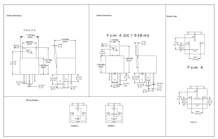
Dimensions in inches with millimeters in brackets below. Tolerance:  $\pm .010$ "
