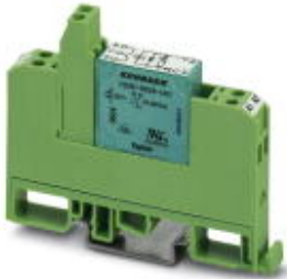
Relay module, with soldered-in miniature switching relay, contact (AgNi): Medium to large loads, 1 PDT, input voltage 120 V AC/DC
