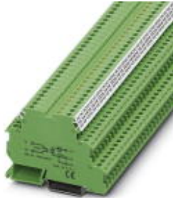
Power solid-state relay terminal block, input: 24 V DC, output: 3 - 30 V DC/3 A, terminal block width: 6.2 mm
