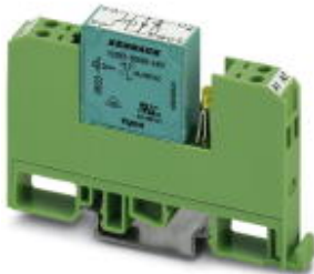
Relay module, with soldered-in miniature switching relay, contact (AgNi): Medium to large loads, 1 N/ C contact, input voltage 24 V DC
