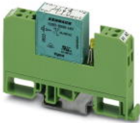
Relay module, with soldered-in miniature switching relay, contacts (AgNi): Medium to large loads, 1 N/O contact, input voltage 230 V AC/DC
