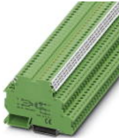
Power solid-state relay terminal block, input: 5 V DC, output: 3 - 30 V DC/3 A, terminal block width: 6.2 mm
