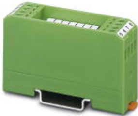
Indicator module, with 7 glow lamps and common return line, input voltage 110 - 230 V AC
