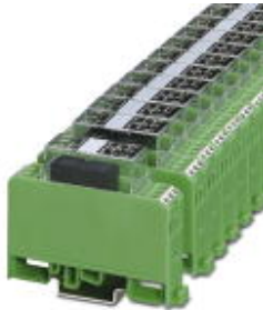
Relay module, with soldered-in miniature switching relay, contact (AgNi): Medium to large loads, double A2 connection, 1 PDT, 120 V AC/DC input voltage
