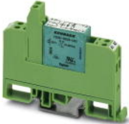
Relay module, with soldered-in miniature switching relay, contact (AgNi): Medium to large loads, 1 PDT, input voltage 24 V DC
