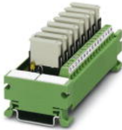
VARIOFACE COMPACT LINE, output module with 8 miniature relays, 1 N/O contact each, plugged, for 24 V DC (incl. relay)
