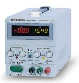
The SPS Series is single output, 360W, switching DC power supply OVP protects SPS and loads from unexpected conditions. High regulation is maintained at 0.01%. Remote sensing adds extra level of precision by compensating cable losses between loads. Turning the output On/Off from external device is available through Remote control terminal. The GPS Series is an ideal solution for power-efficient bench-top or portable applications requiring high regulation.
