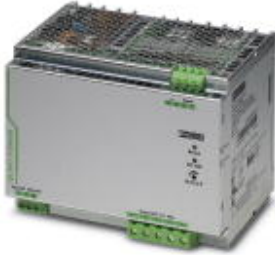
Primary-switched QUINT power supply for DIN rail mounting, input: 1-phase, output: 24 V DC/40 A, with integrated SFB (selective fuse breaking) technology, including mounted universal DIN rail adapter UTA 107
